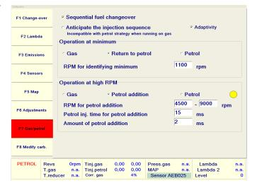
The fact that the system is running on petrol is not indicated on the switch (which stays on gas), but by reading the gas injection time on the computer (which becomes nil).
