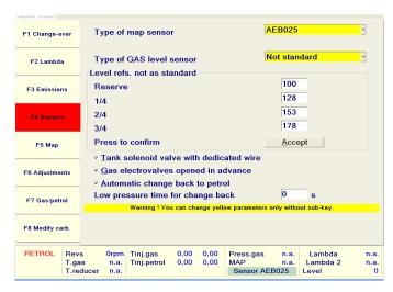
**0 – 90 ohm** – set 0 – 90 ohm if a sensor with output signal sensor ranging between 0 and 90 ohm (e.g. AEB1090) is connected. Refer to the assembly drawing of the gas control unit for connection.
